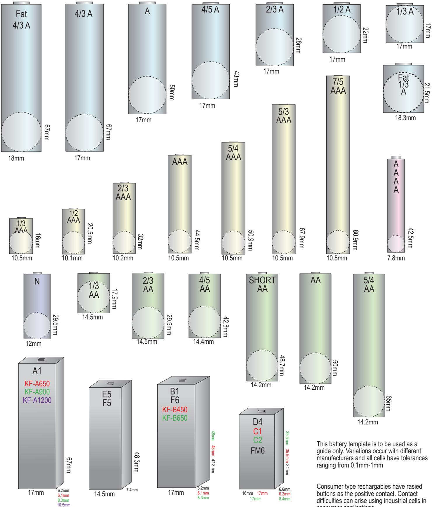
This battery template is to be used as a guide only. Variations occur with different manufacturers and all cells have tolerances ranging from 0.1mm-1mm
